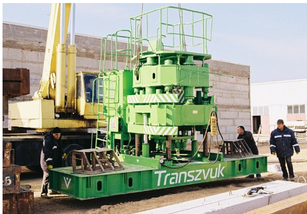
Figure 2. Piling Machine CO-450
